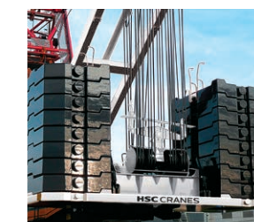
laterally symmetrical counterweight
