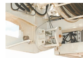
Hydraulically assisted connection pin mechanism (option)
