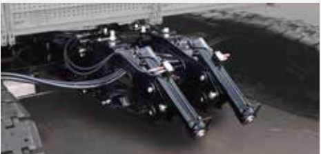
Foldable jack allows work and crawler retraction while mounted OPTION
