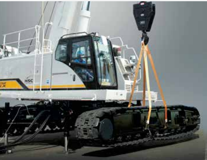
Crawler with self-assembly unit (with crane inspection system) OPTION
