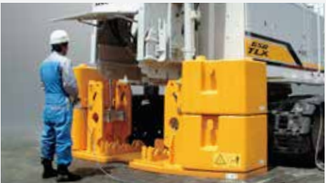
Counter weight with self-assembly unit OPTION
