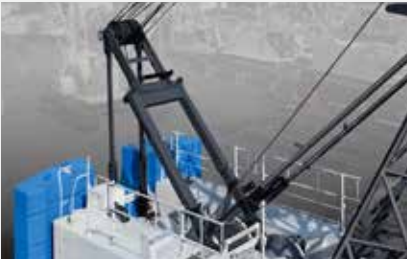
Folding gantry with hoisting cylinder
