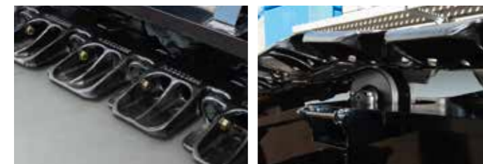
High-durability box type track shoes
