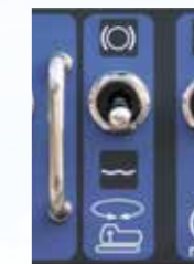
Swing mode selector switch
