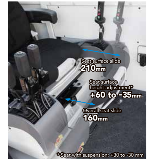
Wide range of seat adjustments
