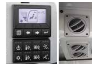
Outside-air intake air-conditioner
