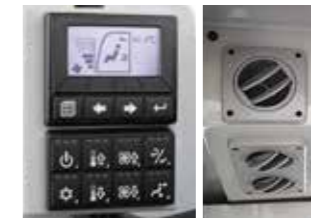
Outside-air intake air-conditioner
