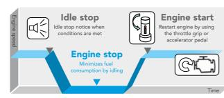
A new auto idle stop function is available for energy-efficient operation and minimal exhaust gas emissions. This prevents unnecessary idling during work to help reduce fuel consumption and limit the level of wear throughout various components. There is no impact on work, as the function stops the engine if the switch is ON and the required conditions are met, and restarts the engine when the accelerator is used.
