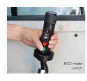
Fuel economy has been improved drastically when winching up and down with light loads. This design ensures energy-efficient operation over repetitive movements or working with loads at heights.
