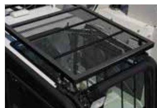
Cab roof window guard The photo is a different color to the standard color (black).
