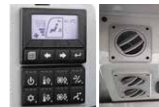
Outside-air intake air-conditioner
