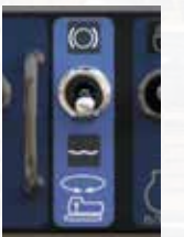
Swing mode selector switch
