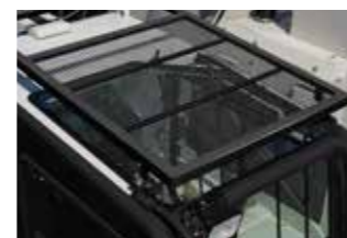
Cab roof window guard OPTION The photo is a different color to the standard color (black).
