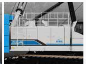
Folding type upper house handrails
