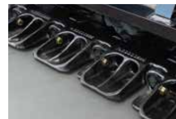
High-durability box type track shoes
