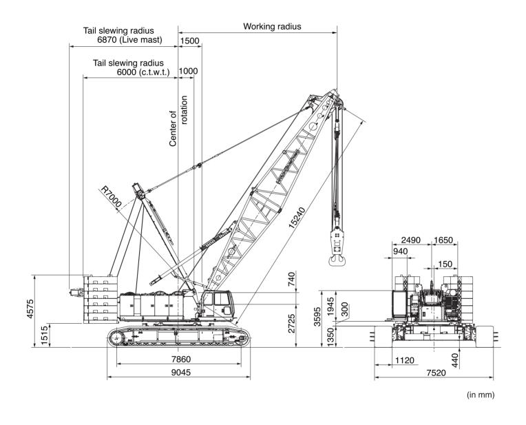
Note: The above general arrangement is under liftcrane application with 15.25m basic boom, and optional 275t hook block.
