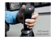
Fuel economy has been improved drastically when winching up and down with light loads. This design ensures energy-efficient operation over repetitive movements or working with loads at heights.
