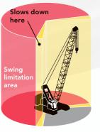
The swing restriction unit prevents the crane from swinging into objects by allowing the swing range to be preset, and notifying the operator of the swing range and automatically stopping the crane when required. Together with the restricted swing range function, the result is an added level of safety when working in
