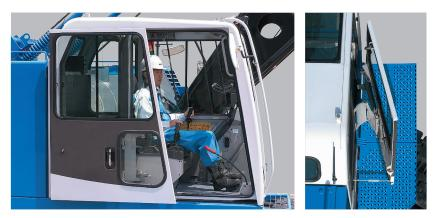
Cab large sliding door with a slewing-link design. For easy entry and exit to and from the cab, and smooth door opening and closing, a slewing-link type large sliding door is designed. And, a slewing-link door design certainly eliminates a troublesome occurrences like a gathering the mud into rail groove, rail-rust and so on unlike rail-slide door.
