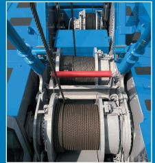
A bigger drum horse power (line pull by line speed) is realized under a new winch drum design with a specially-tailored power increase control system that maximizes engine output under any load condition in whole range of engine
