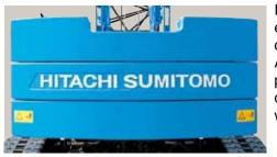
It is able to load boom extension(s) onto counterweight when transport. And, the reversible stack is possible to reduce the time for disassembling/assembling works.
