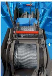
The SCX900-2 is really versatile machine, and certainly performs not only liftcrane/luffing towercrane works but also duty cycle works under clamshell, hammer grab and dragline applications with bigger line pull of 196kN <20t> as maximum with 26 mm dia. cable. In addition, by employing a specially-tailored power increase control, the engine always maximizes its output under any load condition in whole range of engine rpm.
