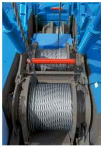
The SCX900-2 is really versatile machine, and certainly performs not only liftcrane/luffing towercrane works but also duty cycle works under clamshell, hammer grab and dragline applications with bigger line pull of 196kN <20t> as maximum with 26 mm dia. cable. In addition, by employing a specially-tailored power increase control, the engine always maximizes its output under any load condition in whole range of engine rpm.
