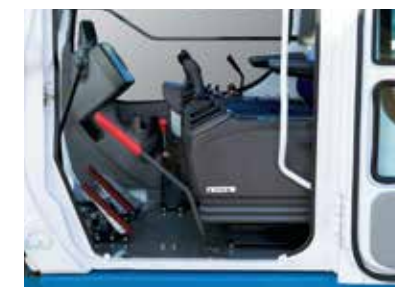
A gate lock lever keeps the crane safe against accidental operations
