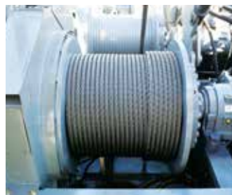
Drum with integrated reduction gear (winch with free-fall function)
