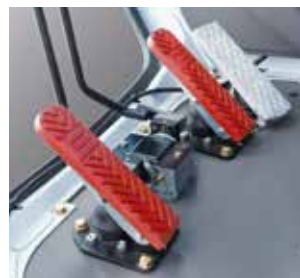
Winch with free-fall function (brake pedals)
