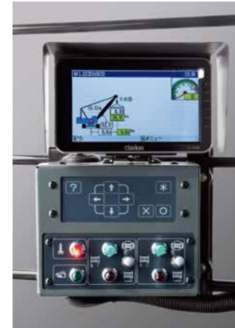
The high-visibility multifunctional moment limiter can be set easily with an interactive interface
