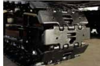
High-durability flat shoes to minimize road damage (optional for SCX550E)
