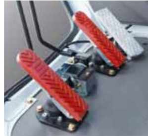
Winch with free-fall function (brake pedals)
